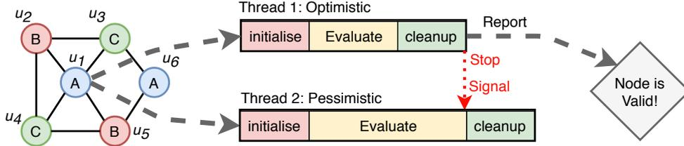
Figure 5: The two-threaded PSI solution
