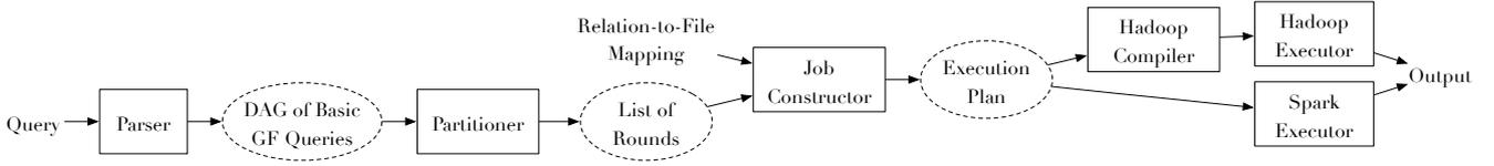
Figure 1: The GUMBO workflow.
